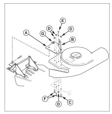
Figure 5. Assemble Turbo
